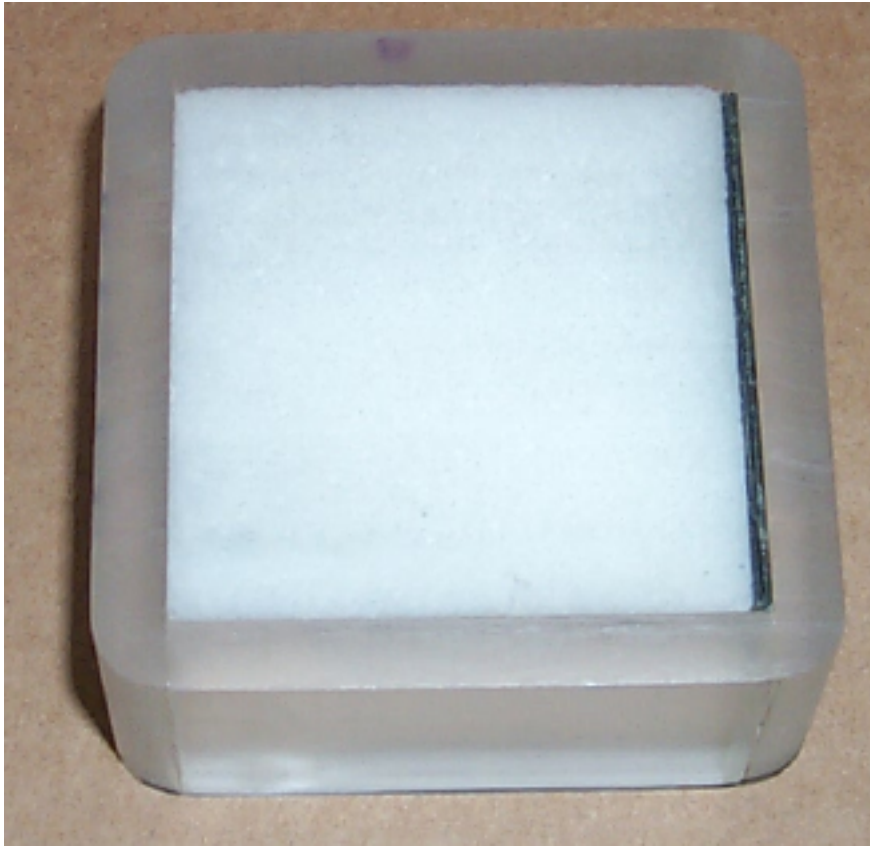
Figure 2. Photograph of 2"-wide by 2"-long by 1.1"-deep sample (includes 2 0.059"-thick shims)
